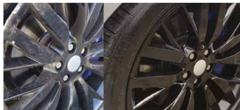
Scraped curb rashed wheel before and after 30 min of repair time
