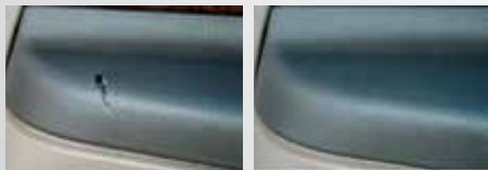
Interior tear in armrest before and after 60 minutes of work.
