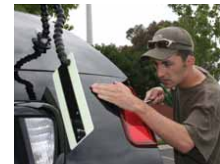
Technician using Dent Board while removing a dent.
